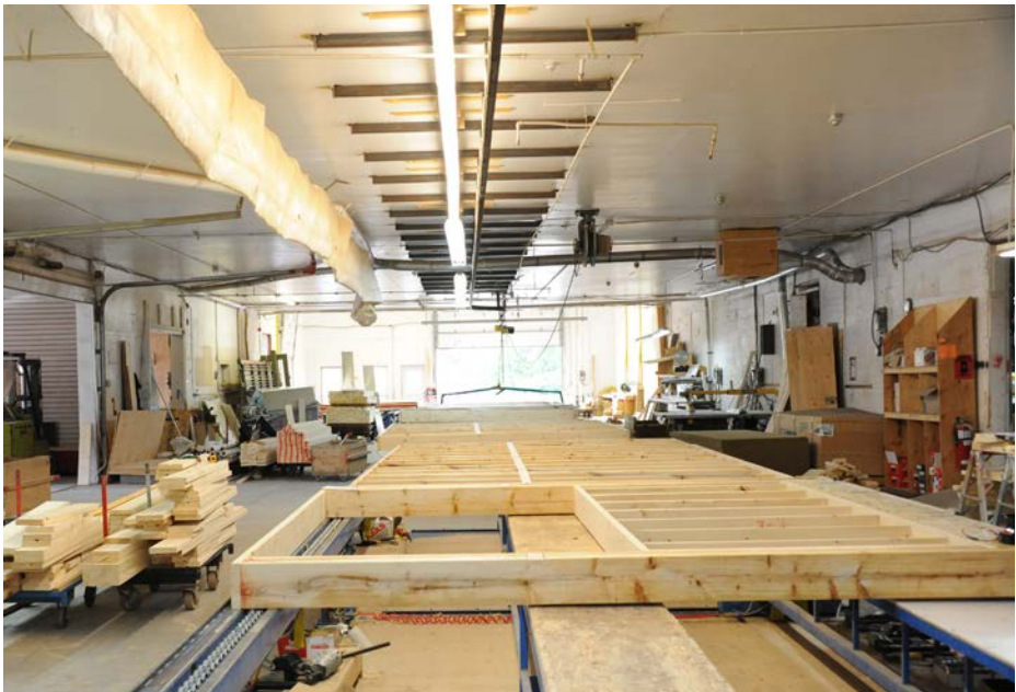
Wall Panels Built in a Factory
